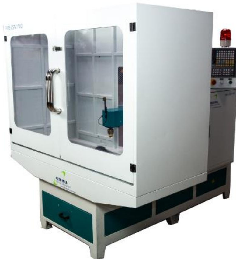
Figure 4.1.1 Countersink machine FME-CSA-1100
